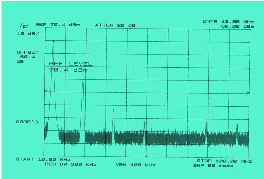
Figure 12: RF Output Spectrum, 1KW Output Power
