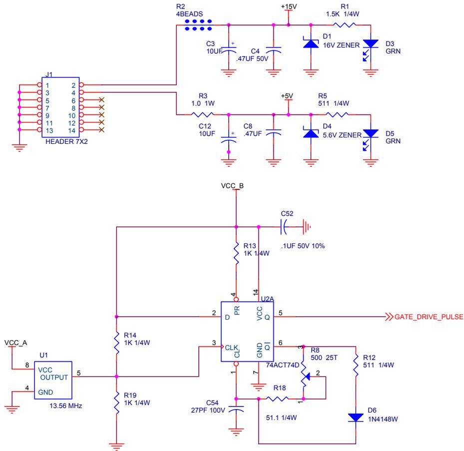
**Figure 2: PRF-1150 DC and Gate-Drive Schematic**
