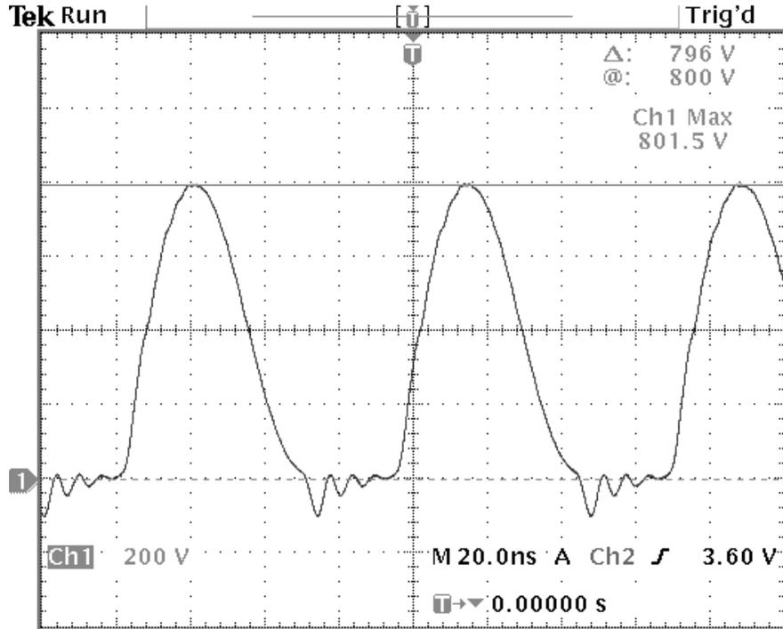
Figure 10: Drain Waveform @ U3, Drain, 1KW output power
