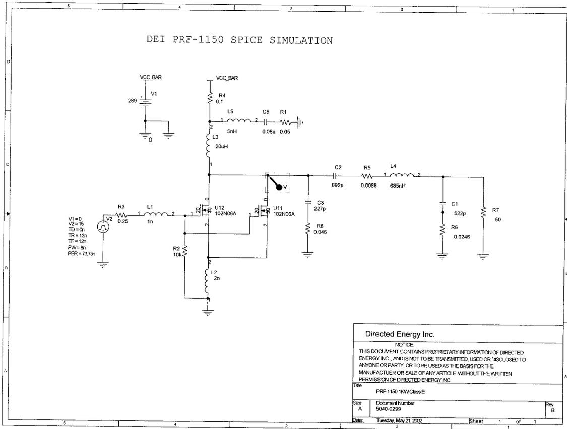
Figure 14: PRF-1150 SPICE Simulation Circuit
