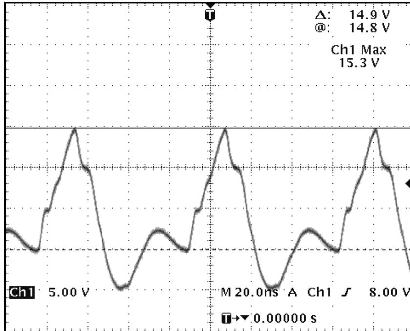
Figure 9: Gate Drive Pulse at U3 gate
