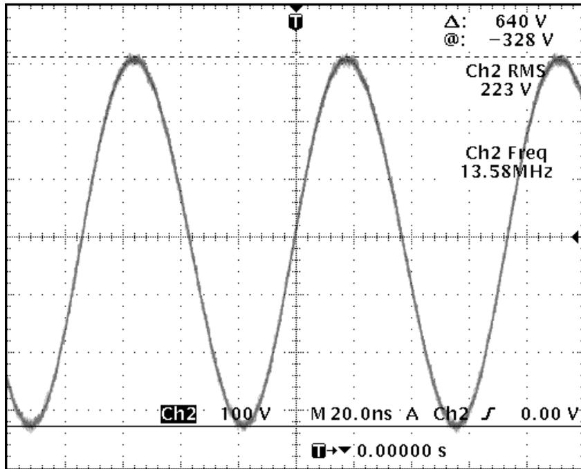
Figure 11: RF output Waveform J2, 1KW output power
