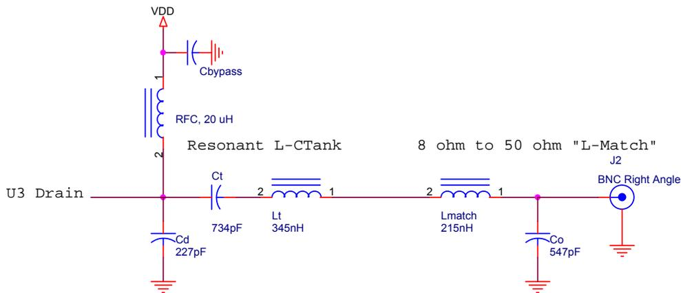
Figure 9: Simplified Output Tank and L-Match Schematic
