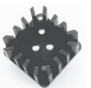
Achieve optimum natural convection cooling per unit volume occupied above the printed circuit board for TO-3 (one semiconductor package per heat sink) or for two TO-220 style cases, when this low-cost heat sink is used. Any mounting attitude will provide free circulation of air in natural convection applications. These 680 Series heat sinks can also be specified without any semiconductor mounting hole pattern by specifying suffix "K" (Example: 680-5K).
