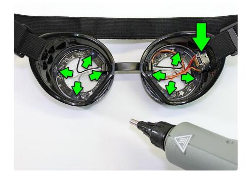
PRO TIP: if you used hot glue and need to remove the rings later, dip a Q-Tip in rubbing alcohol, touch it to the edge of each blob of glue and allow it to soak in for a few seconds. This doesn't dissolve the glue; it seeps between the two parts and cleanly breaks the bond. The glue should peel away with little effort. Science!
