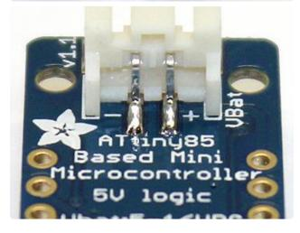
Start by "tinning" one of the JST pads on the back of the Trinket...heat the pad and apply solder so the whole surface is coated.
