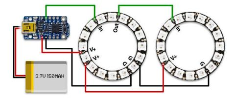
This diagram uses the original Trinket but you can also use the Trinket M0 with the exact same wiring!
