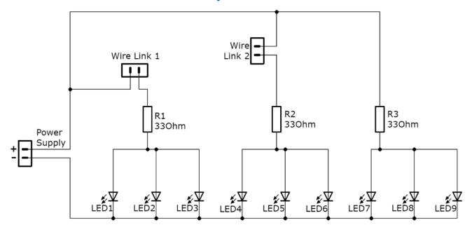
The circuit diagram for the 5V LED Desk Lamp is shown above. It is a very simple circuit. The board contains nine LEDs, these are grouped in threes, with each group of three sharing a current limit resistor.
