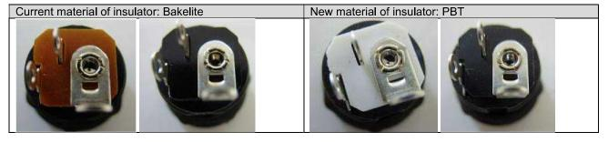
Change of insulator plastic material from Bakelite to PBT with glass.
