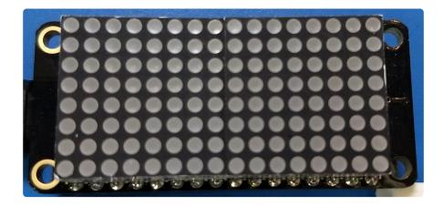
By default the display will update automatically. This way you do not need to call the s how function every time you update the display buffer. However, this means it is being sent the contents of the display buffer with every change. This can slow things down
