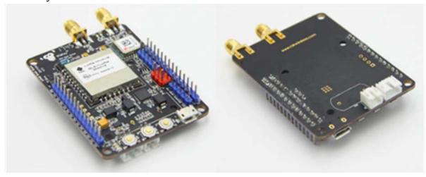
The RAK815 (RAK813 LoRaB Breakboard) includes beacon location for indoor and GPS location for outdoor as well as five kinds of sensors for various applications for the LoRa network. It adopts the latest LoRaWan 1.0.2 protocol and latest Bluetooth 5.0 protocol. It also supports LoRaWAN Node mode and Bluetooth transparent transmission. It also has built in GPS, acceleration, temperature and humidity sensors, and expanded I2C LCD interface.
